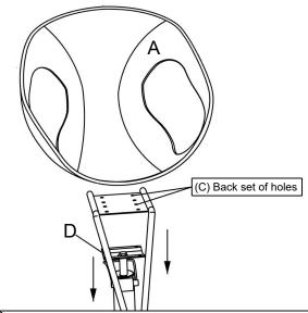
1) Secure the base, bracket (D), and footrest (C) to the chair top (A) with 4 bolt/washer sets (E) as shown below. \*Pump the hydraulic up higher if necessary to see underneath
