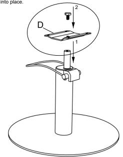
1) ! SEEK HELP TO DO THIS STEP! Two extra sets of hands are best to help keep everything in place. Once help is found, align the chair bracket (D) to the FRONT set of holes on the footrest bar (C). Next, locate the holes found underneath the chair top (A) and hold in
